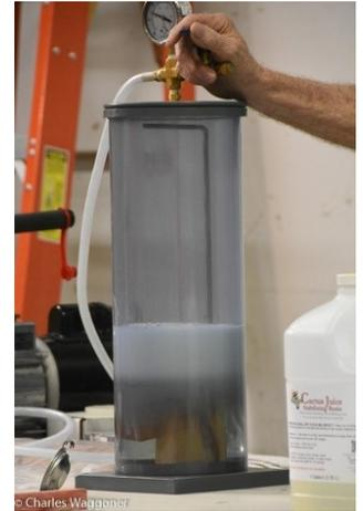
At this point I disconnect the venturi and slowly open the chamber relief valve.
